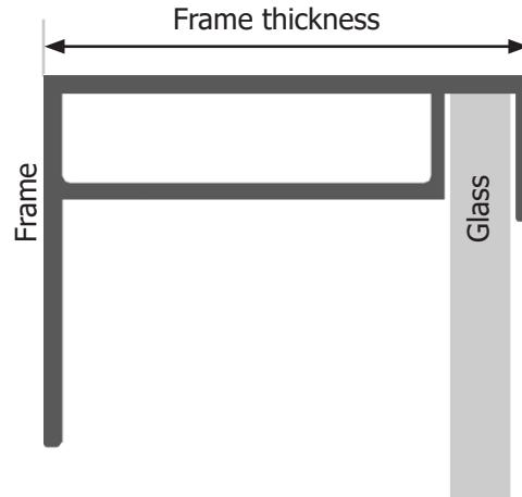
If frame thickness is ≤35mm (1.4in), install with the TS4 label facing the PV module.
